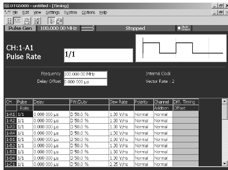
Figure 4-5: Timing window (Pulse Generator mode)
